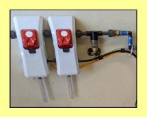
The AccuMAX accurately dilutes dip at the push of a button. No electricity is needed... just a water outlet (20 psi). Water moves through the venturi pump system pulling the correct amount of concentrated product through metering tips to make RTU Product. It is great for filling dip cups or gallon jugs.
