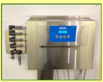
The Knight system has a micro processor based digital blending controller which allows you to use different teat dip concentrations. It has high reliable electric diaphragm pumps which allow it to deliver precise fluid volumes based on flow meter signals and formulation composition. It also has a SD card which allows you to retrieve usage reports.
