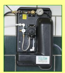
The Parlor Master accurately dilutes and delivers product to the parlor with one convenient unit. No electricity is needed... just a water outlet (20 psi) and compressed air. This pump has a float inside and regenerates product as it is depleted, leaving fresh product. Metering tips are used to insure the right amount of concentrated product is used.
